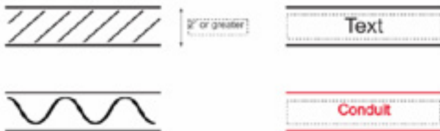
Figure 1: Samples of proper markings of embedments
